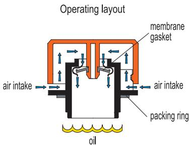
The membrane gasket warps and lets air inside the reservoir due to the effect of the vacuum which is created by the liquid discharge.
