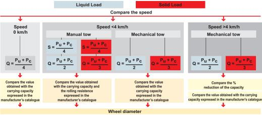
$\mathbf{S}$  = rolling resistance  $\mathbf{Q}$  = load capacity  $\mathbf{P}_{\mathbf{U}}$  = weight to transport  $\mathbf{P}_{\mathbf{C}}$  = equipement weight
