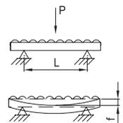
P: applied in the centre of the roller track, the load value generates an elastic deflection of the aluminum profile beyond which the product functionality may be compromised. At this load value, however, no permanent deformation of the material occurs.
