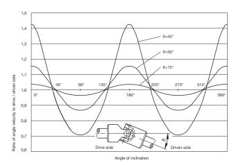
The single universal joints transfer the initial smooth rotation as an irregular rotation. One revolution of the drive shaft via single universal joint will cause the driven shaft to accelerate and decelerate twice. The extent of the irregularity depends on the operating angle  $\beta$ .
