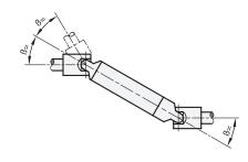
For a smooth transfer of a rotating speed, the angle of inclination  $\upbeta$  must be equal at both ends of the connecting shaft.
