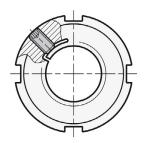
Slotted nuts are always indispensable whenever the axial interplay of shafts, bearings or spindles needs to be adjusted. Elesa+Ganter has now found a particularly elegant way of solving the problem of securing against rotation.
