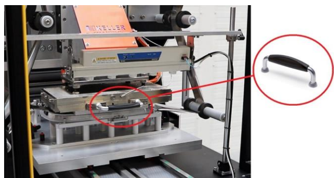
Application of MMT. handle on the HS K-Desk Precision machine
