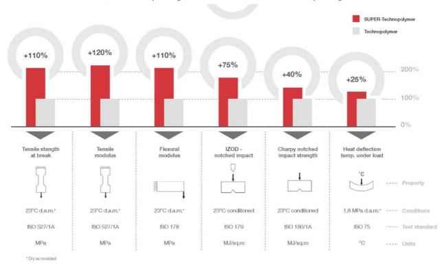
Comparison of Mechanical Properties between SUPER-Technopolymer and Technopolymer
